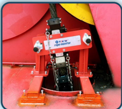
Floating Crane Wire Rope Inspector
