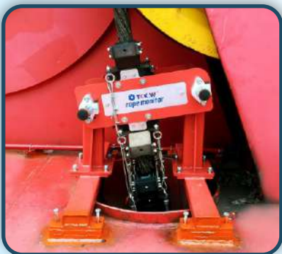
Floating Crane Wire Rope Inspector
